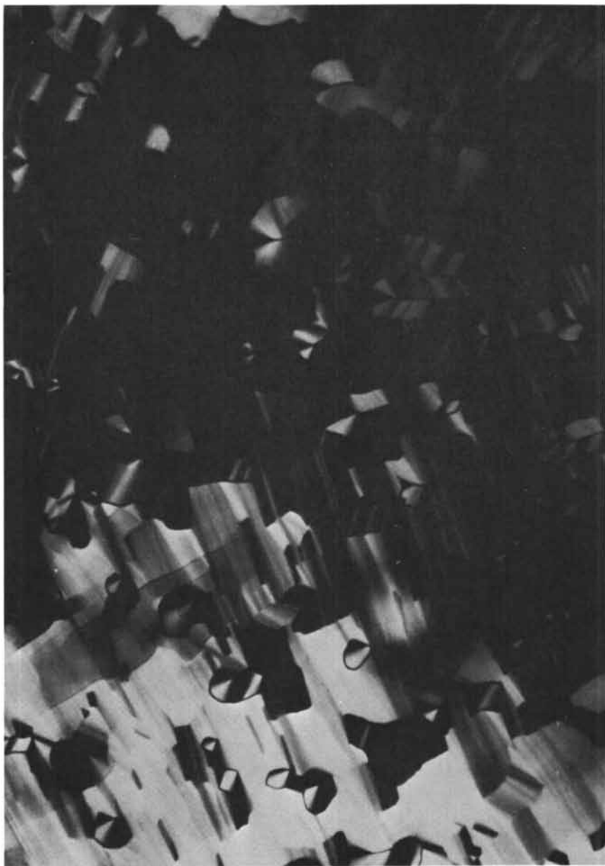
Figure 4. Photomicrograph at 298°K of 90/1 molar ratio \text{CH}_3\text{OH}/ bis(2-ethylhexyl) sodium sulfosuccinate; magnification 330X; crossed polaroids.
